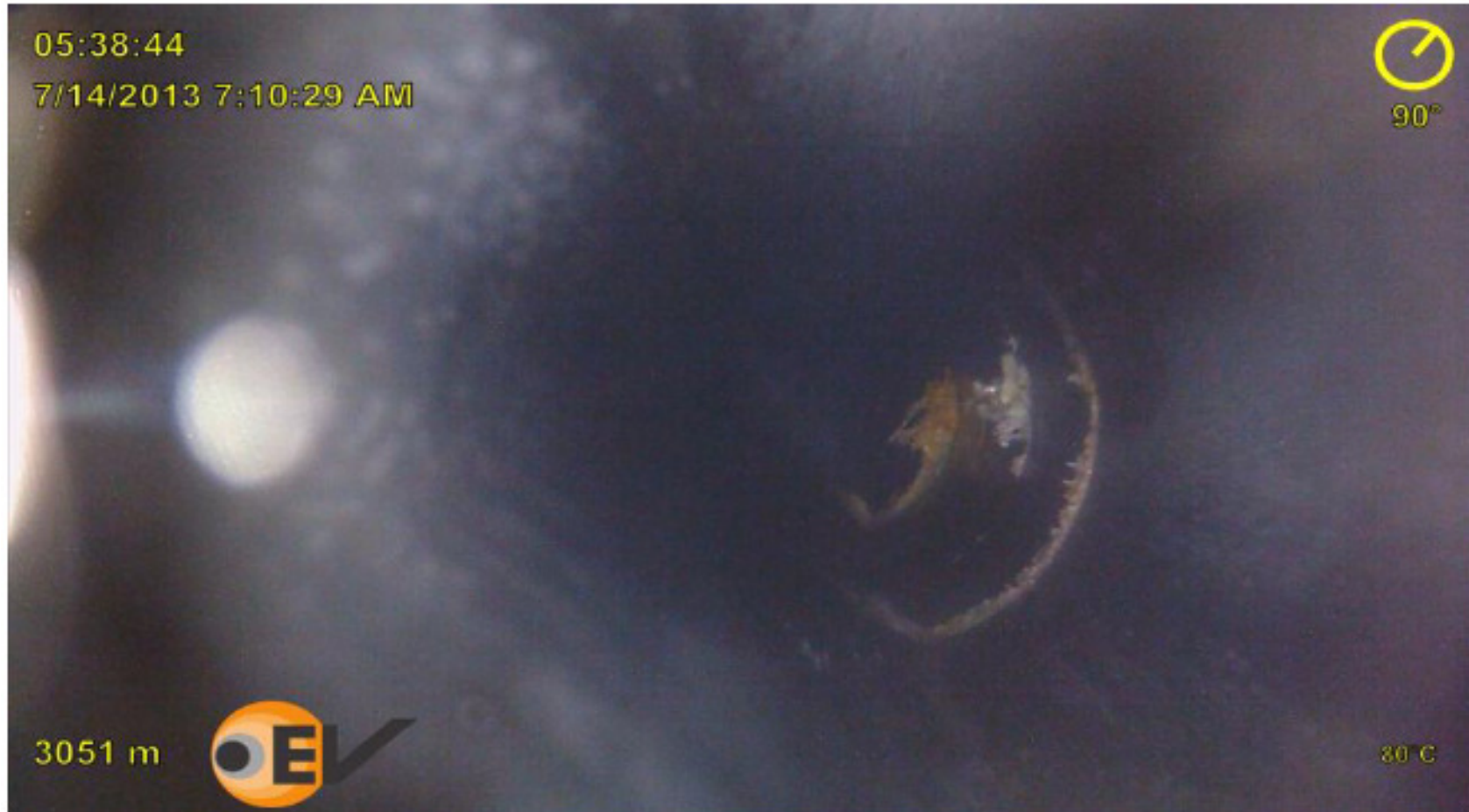
Figure 9 – Perforations with minimal cooling
